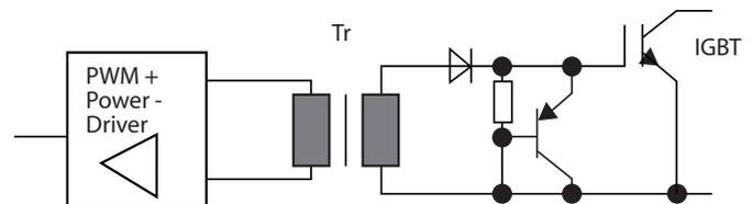
Drive transformer (Signal) + Drive transformer (Power).
